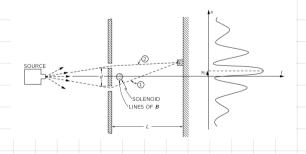
Shift in the interference pattern: Now consider the addition of a very time (ittg-bitty) solemoid in the region enclosed by the paths of the two electrons.
