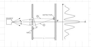
Interference: Consider electrons 1 and 2 with amplitudes  $C_1e^{i\theta_1}$  and  $C_2e^{i\theta_2}$  respectively. The interference pattern will depend on the relative phase between the two electrons i.e.  $S = \bar{x}_1 - \bar{x}_2$ . Why?
